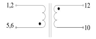
Primary windings to be connected In parallel on the PC board.
